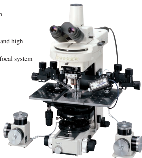
Configuration with Narishige micromanipulators and epi-fluorescence attachment
