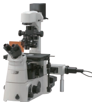
Ti-U configuration with epi-fluorescence illuminator
