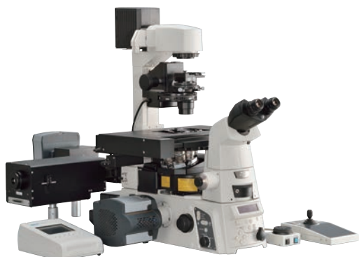
Ti-E configuration with motorized accessories
